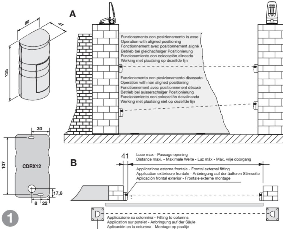
**INSTALLAZIONE CON FORATURA MURO - INSTALLATION WITH THROUGH THE WALL WIRING**
